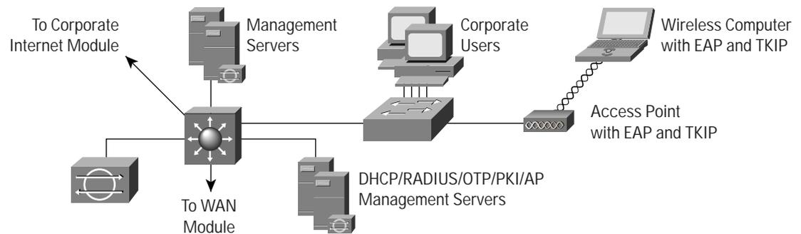
EAP access in the medium WLAN design has wireless access points connected to the existing Layer 2 access switch in the medium-campus module. RADIUS and DHCP servers are also located in the campus module, but off a distinct Layer 3 subnet on the central-campus Layer 3 switch. The wireless EAP users will require DHCP and RADIUS authentication services to access the medium-campus network. If the medium network is a branch office, the DHCP and RADIUS servers may reside at the corporate office.
