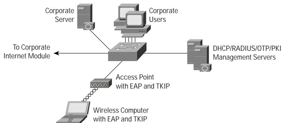
Cisco EAP access in the small WLAN design has wireless access points connected to the existing Layer 2 access switch in the small-campus module. The wireless EAP users require DHCP and RADIUS authentication services to access the small-campus network. Because of the single-site nature of small networks, the RADIUS and DHCP servers reside locally connected to the Layer 2 switch in the campus module.
